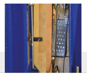
Experimental data on the static performance of a timber-to-steel connection with ALADIN interposed
